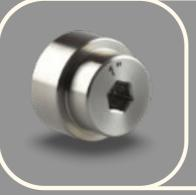
This 1 inch yoke nut socket fits on Oceanic, Hollis, Aeris, Dive Rite, and more yoke (INT) first-stage regulators. On this tool located at the top of the socket is an 8mm hex connection which is easily accessible with an 8mm long hex key with a connection to a 3/8" socket wrench.
